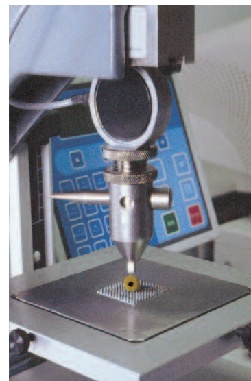
Figure 23 - Measure of a kibble's resistance to pressure
